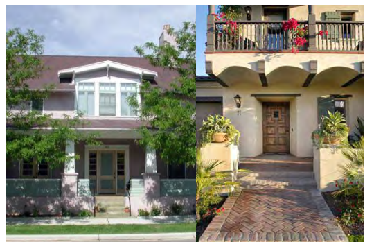
Recessed entries, windows, roof, column/stairs and balconies help emphasize the entry.
