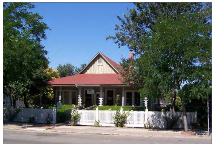
Porch Example - small setback with or without fence and raised porch create separation from street while providing an entry feature and outdoor living area for the dwelling.
