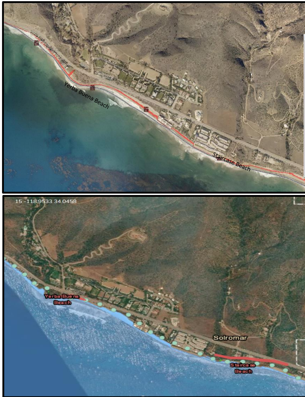
Figure 2-15. Tidal inundation along the Solromar Existing Community area with approximately 5 feet of sea level rise. The red lines represent potential bluff erosion. Results of sea level rise as modeled by Coastal Resilience (top) and CoSMoS (bottom).
