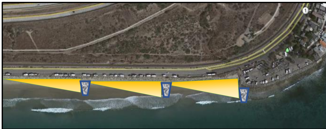
Figure B-6. Map view of cross-shore cobble groins with retained sand on the Rincon Parkway and at Faria County Beach Park (not to scale).
