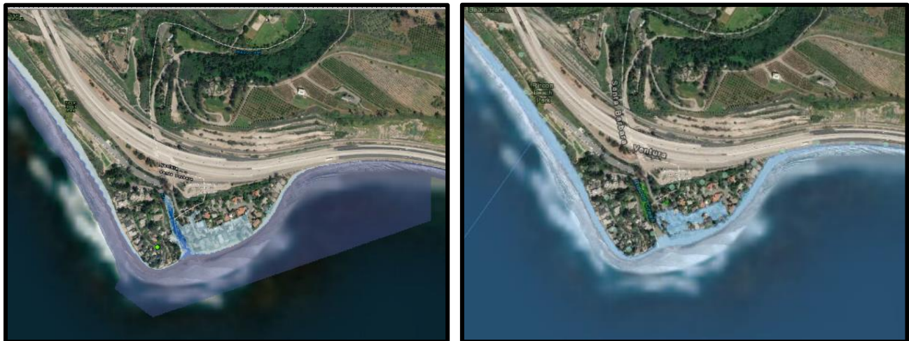
Figure 2-2. Tidal inundation with about 5 feet of sea level rise at Rincon Point according to Coastal Resilience (left) and CosMoS (right).
