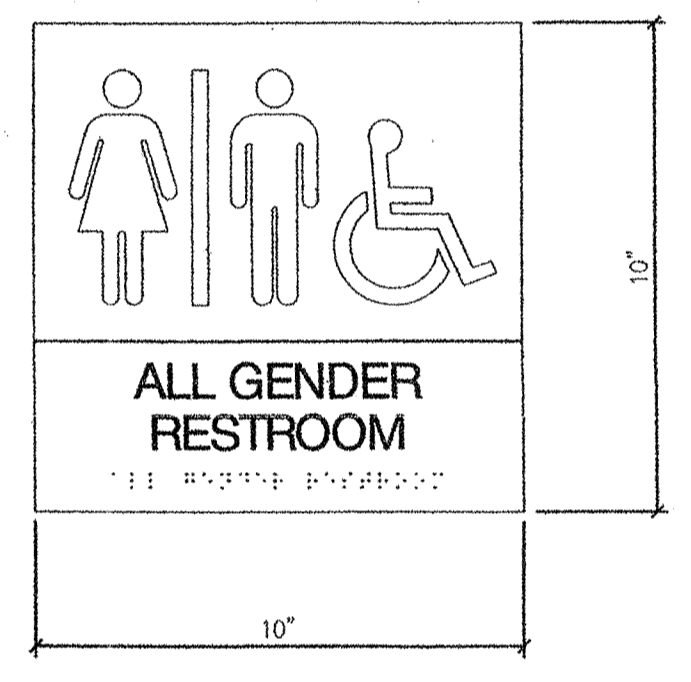
DETAIL 3 ACCESS ALL GENDER WALL SIGN N.T.S.
